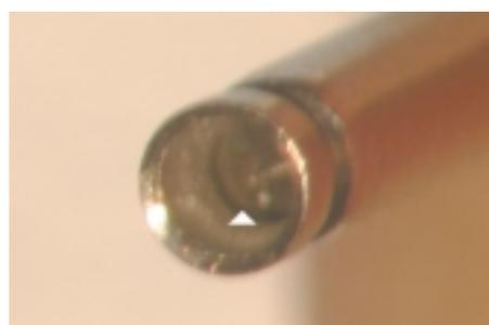
**Figure 4.** The tip of the Masserann extractor.
