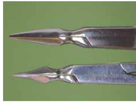
Figure 8. Steiglitz forceps before and after modification on a prosthetics lathe.
