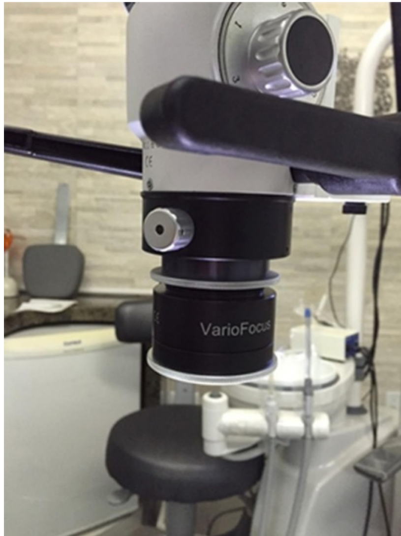
Figure 8.2 Vario Focus da JC-Optik, It Allows focus between 200 and 300 mm.
