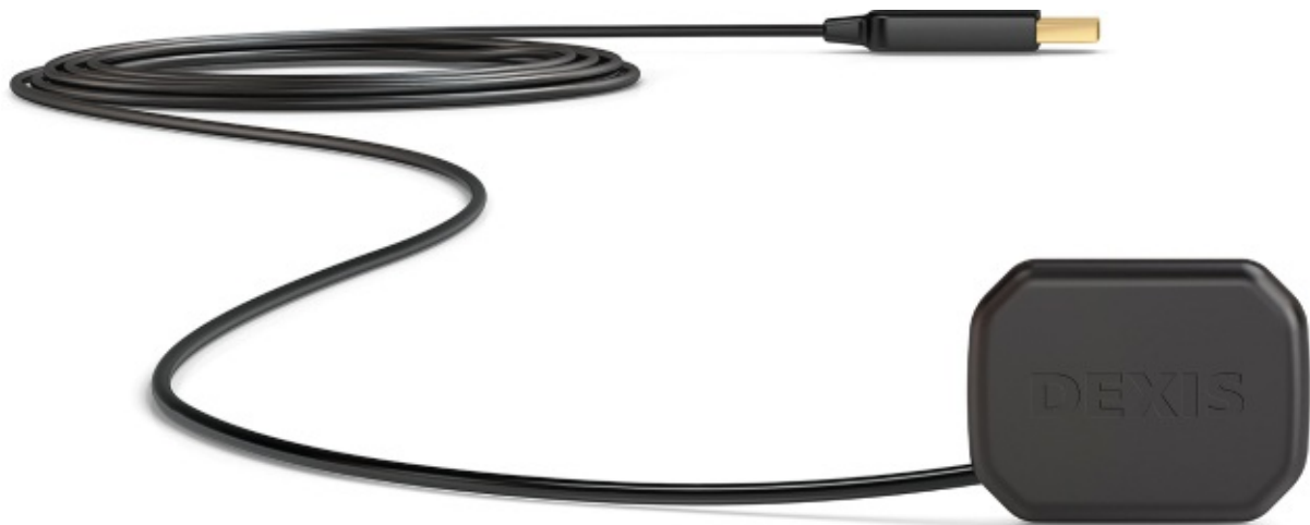
Figure 2.2 The Dexis Platinum Sensor features a beveled corner design to enhance patient comfort. The attached wire connects to a computer via USB to yield high-resolution images instantly.
