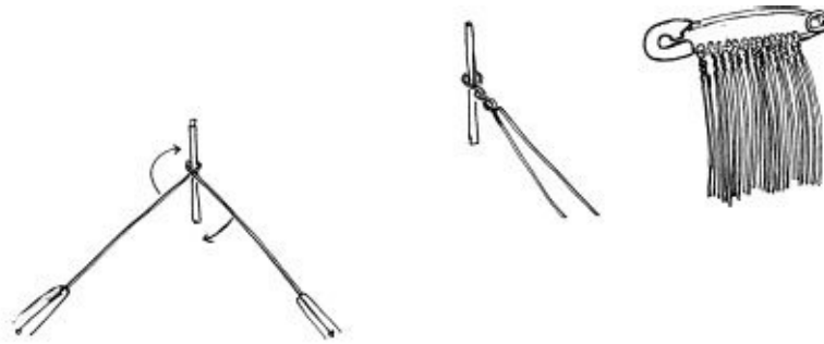
Figure 8.6 Making eyelet wires from 0.5 mm stretched stainless steel wire.
