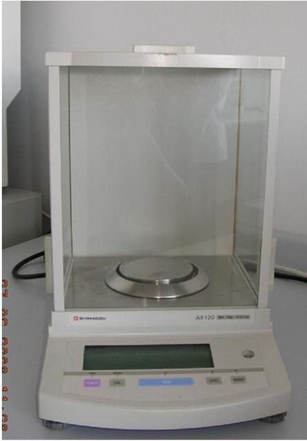
**FIGURE 1.** Photograph of the fine electronic weight measurement device used in the present study.
