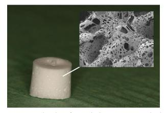
**FIGURE 1.** Polyurethane foam with electron microscopic detail showing interconnected pore structure.
