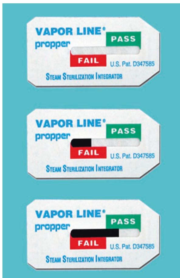
Photo 2.1 Example of a chemical multiparameter integrator (courtesy of Vapor Line)
