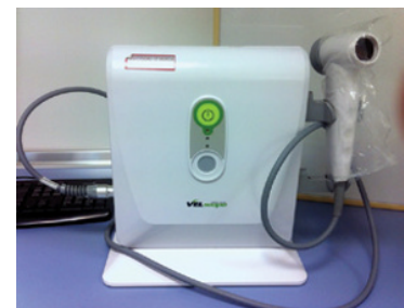
Figure 2.6 Fluorescence spectroscopy system (Velscope).
